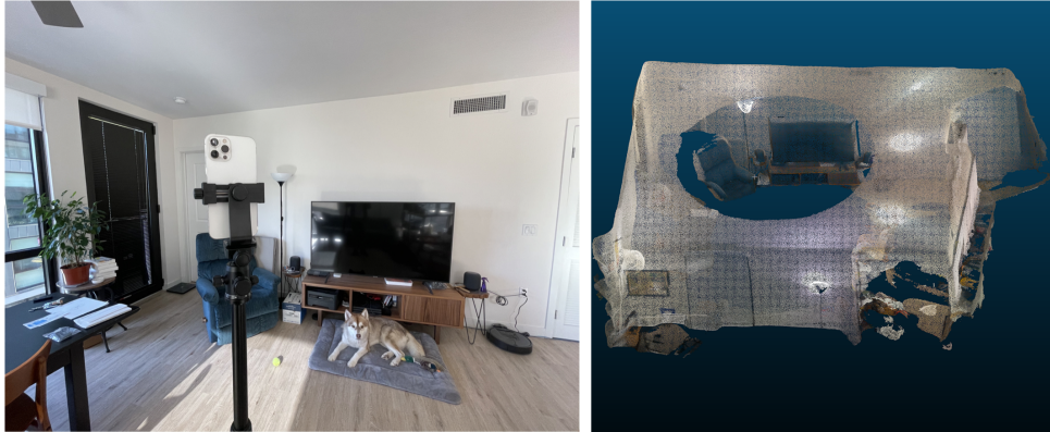
Figure 1: Tripod mounted iPhone 12 Pro with LiDAR sensor (left) which can be rotated freely during scanning. The point cloud scene of the living room (after centering and processing) visualized using CloudCompare.
